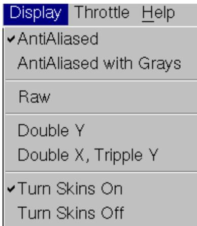
**Anti Aliased:** This is the normal mode you should use with the Lisa Office System. This corrects the square pixel issues and uses anti-aliasing to fix most artifacts.
