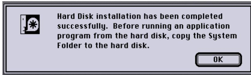
The install is complete, but you must copy the system folder to the hard drive, otherwise attempting to boot from it will cause a Sad Mac error.
